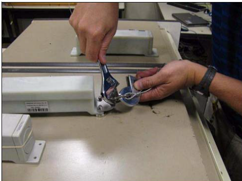
Figure 5-5: Tighten Threaded Link with Two Crescent Wrenches
