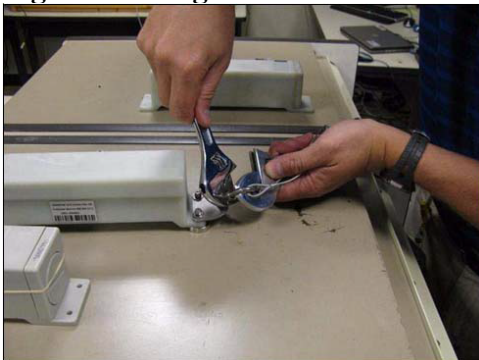
Figure 7-4: Tighten Threaded Link with Two Crescent Wrenches
