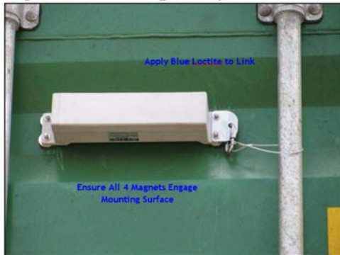
Figure 7-3: Wrap Lanyard around Locking Rod and Secure with Threaded Link
